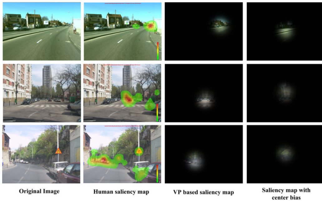
Figure 8. Comparison of the center bias model and our proposed model in the curved road environment.
