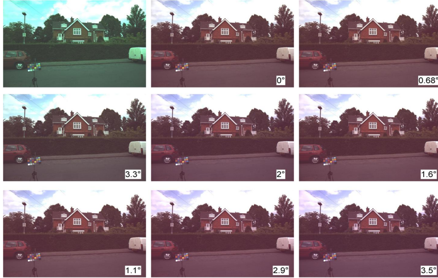
Fig.2. The result of an image of the Gehler-Shi dataset, from left to right and from top to bottom represent respectively the original image, ideal image corrected by ground truth, estimated image corrected by Our method, Grey world, White patch, Shade of grey, General of grey, Grey edge of first order, Grey edge of second order. The corresponding angular errors are shown in the lower right corner of the images.
