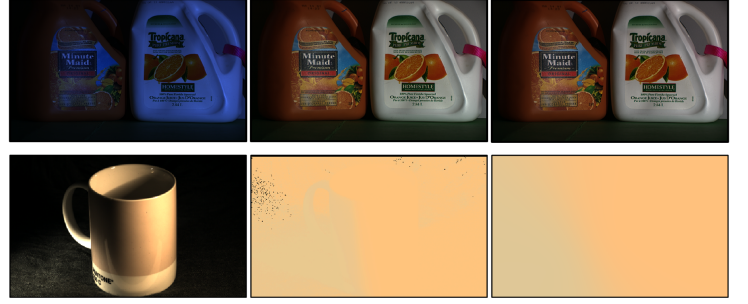
Figure 1: The top row lists (from left to right) the original color-biased image under single illuminant, the ground-truth image, and the corrected image by the proposed method. The bottom row shows an example of multi-illuminant estimation; from left to right: original image, ground-truth illuminants, and the estimated illuminants in this paper.
